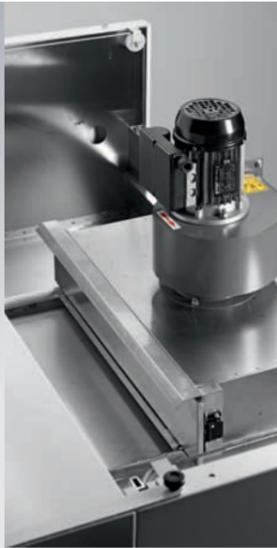
1. stainless steel fume cabinet with air extractor fan with metallic filter and arrangement for active carbon filter (GK2)
